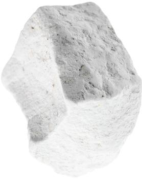
Opaque, electrical and thermal insulator, soft (for rock), rough, rigid, slightly absorbent
