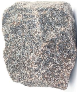
Opaque, electrical and thermal insulator, hard, rigid, rough, waterproof
